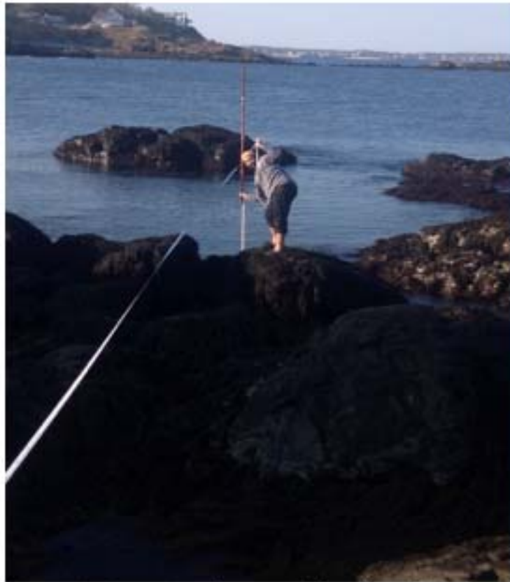
Picture 1: Measuring the vertical height of the reference point at the time of low tide. October 26 th , 2012 at Northeastern Marine Science Center, Nahant, MA.
